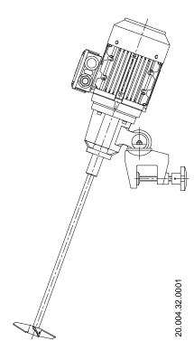
The design of the gag, with a swivel ball and socket joint, allows for a triple mixing action. Fixing the agitator with the correct angle for the required mixing is instantaneous and a tried and tested mixing result can be recorded and reproduced with the three positions. See the following figure:
